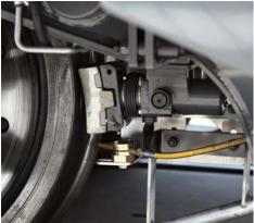
bogie wheels wheel flanges ester oil with bentonite thickener and solid lubricant
